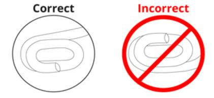
• Make sure that the cut end of the **EZ-Splice**® strand is on the bottom.
