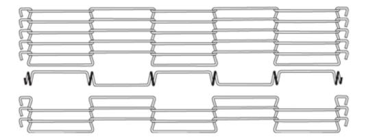
• Once both ends of the belt are aligned with the spaces in the **EZ-Splice**® strand, turn the **EZ-Splice**® strand over and hook both end loops in as shown below.
