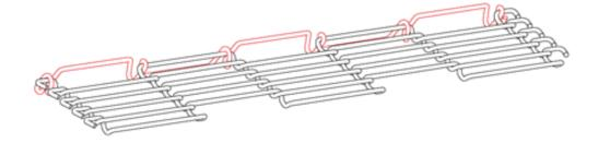
• Once the bottom half is all locked into the appropriate spaces across the width of the belt, turn the **EZ-Splice**® strand about 1/4 of a turn or about 90° up as shown.
