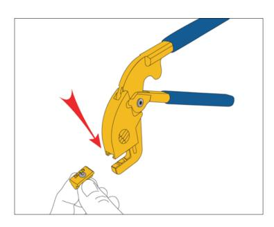
• Insert the beveled edge of the bit into the jaw slot, pushing in with your index finger until you hear a click indicating that the bit is locked into place. Make sure to use the correct bit that matches your belt.
