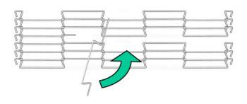
Now insert the short end down through the 4<sup>th</sup> space on the lower end of the belt and up through the 3<sup>rd</sup> space in the upper belt end (use pliers if necessary). Then straighten the strand section.
