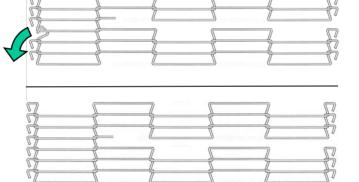
Straighten wire with pliers or wire straightener. The first stage is completed.
