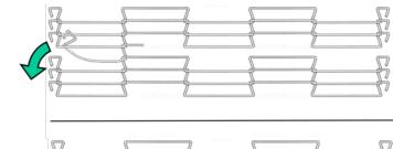
With pliers take the lower edge loop and hook it up through the first space to loop the edges together.
