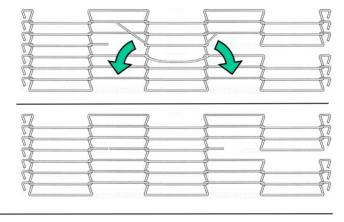
With the last space place the long end of the cut wire section down through the  $4^{th}$  space on the lower belt end and up through the last  $(5^{th})$  space on the upper belt end. Turn the wire section anticlockwise into the spaces to lock in the Z-bend link assembly.
