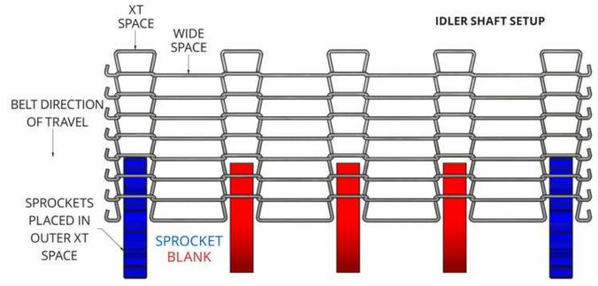
In setting up the idler shaft, install one drive sprocket per outside XT space of your belt (figure above). Then, install one blank on each of the inside XT spaces across the width of the belt. Make sure to fully secure each component along the shafts.
