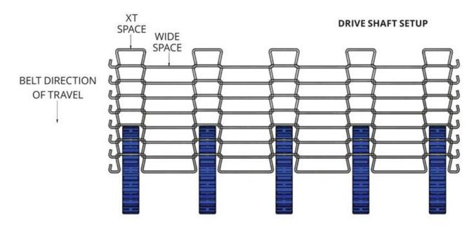
To setup the drive shaft, install one drive sprocket per XT space along the full width of the drive shaft (figure above).
