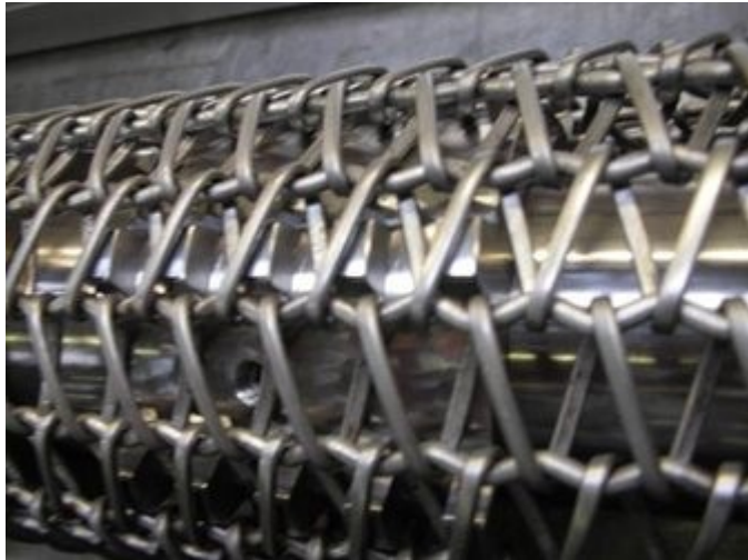
Typical Drive Shaft Set-up with Balanced Spiral Flat Wire Belting and Bi-Directional Sprockets.
