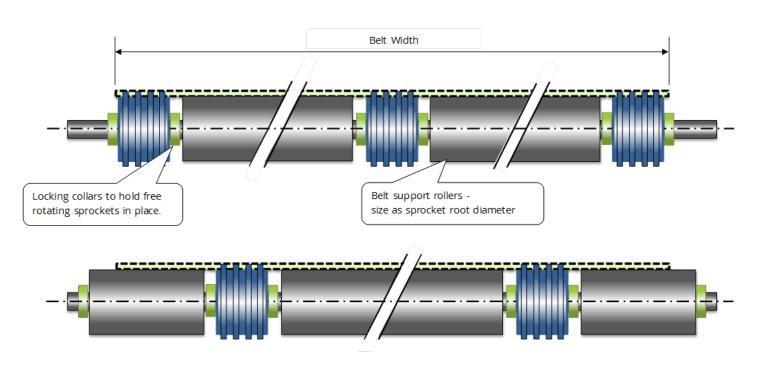
Belt circuit should be arranged such that there is sufficient wrap around the sprocket to ensure that the teeth remain engaged with the mesh.
