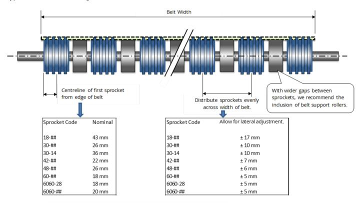
Suggested Tracking Shaft (Transfer or Idle Shaft) Optional Arrangements:-
