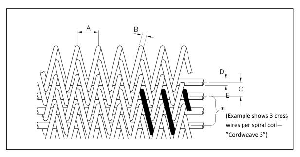
\*\*NOTE: When measuring pitch, it is best practise to measure over 10 pitches and divide by 10 to obtain the average pitch.
