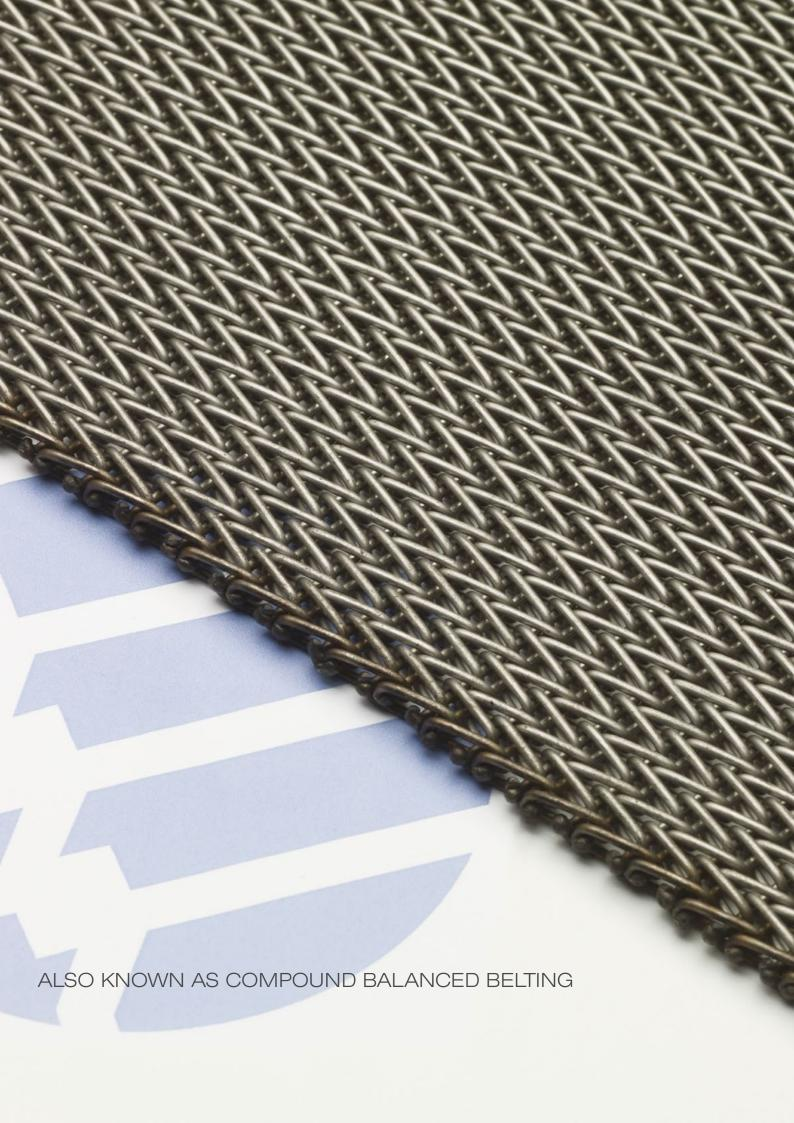
Cordweave belts offer an extremely close and flat mesh for applications where very small items are being conveyed. Cordweave also provides a uniform heat transfer across the belt due to its high density and smooth carrying surface. These characteristics make Cordweave a popular choice in a wide variety of applications, ranging from biscuit baking to sorting small mechanical components.
