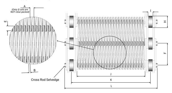
**\*NOTE:** When measuring pitch A it is best practise to measure over 10 pitches and then divide by 10 to obtain the average pitch.
