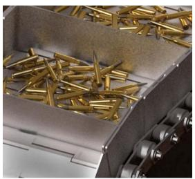
All available specifications can be supplied with side plates and cross flights in various combinations of height and design enabling elevation or product separation as required by the application.
