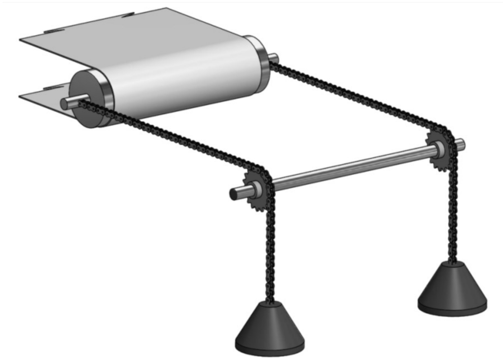
Gravity weighted chain sprocket arrangement (sprockets keyed to shaft).
