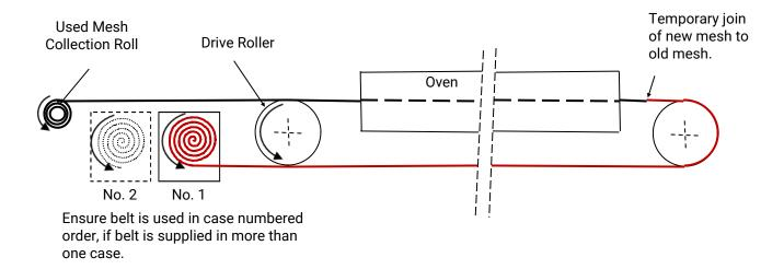
Once the new belt length exits the oven at the discharge cut off the temporary join of the old belt to the new belt. Roll up the remaining old belt onto the spindle for re-cycling. Then pull the remaining new belt from the box and lap the trailing end up around the drive roller to meet the leading new belt end. Pull and stretch the belt by hand with as much force as you can to remove any slack in the belt so both ends meet.
