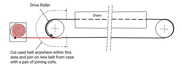
Then pull top surface cut belt end by hand or other mechanical assistance through the system at the same time unrolling new belt from the case. The old used belt can then be rolled on to a collection spindle for disposal.
