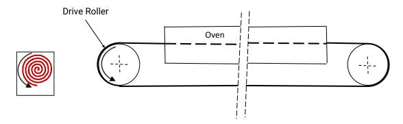
Ensure that all belt tension is released by adjusting to the minimum stop position the belt take-up mechanism.
