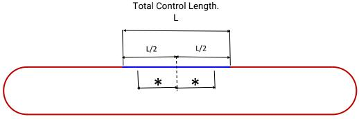
\* Maximum cutting length for belt shortening = 75% of length L/2. Only shorten belt here upon installation and on any necessary future occasions. When belt is supplied in multiple cases only shorten belt at final join ends marked "1".
