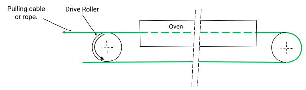
Then open the new belt case (or case no. 1 for multiple cases) to check the band running direction, as noted on a plastic label attached to the belt. Position the case at the drive discharge end of the conveyor as shown below.
