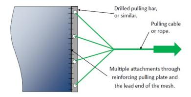
Then pull the belt through the circuit using the cable/rope. DO NOT allow the belt edges or lead of the belt to contact or catch on any part of the frame or system. If necessary guide the belt by hand. Irreparable damage to the belt will affect the correct belt running and may result in early failure.
