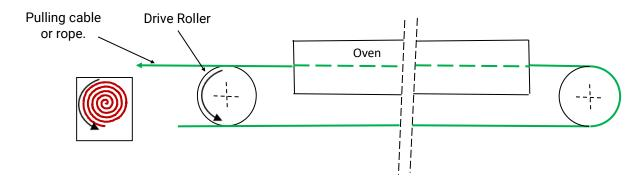
Attach to the leading edge of the belt in multiple places across the width a reinforcing pulling bar. Then attach the pulling bar to the cable/rope as shown below.
