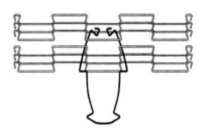
Whilst Wire Belt offers many innovative belt joining methods such as EZSplice™ and join clips, there are many applications where only a full strand weave is appropriate. Full strand weaving is a joining method where a single strand is woven through the leading and trailing end of the belt to create a join. This method is very popular with coating and enrobing applications since belt strength is maintained and the carrying surface uninterrupted.
